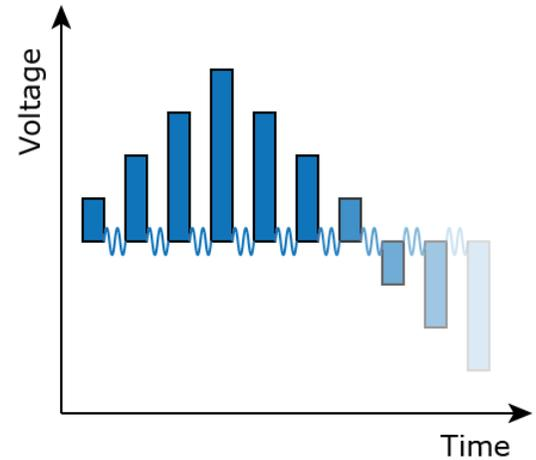
Figure 8: Sketch of the voltage during the hysteresis cycle. The DC pulses are applied to switch the domain while the PFM mode detects the phase after every pulse to measure the orientation.
