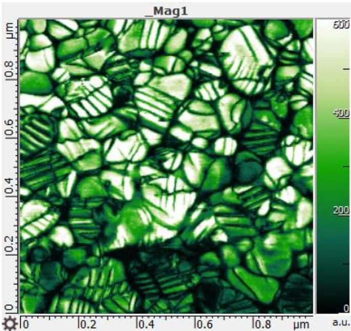
Figure 4: Amplitude of the lateral piezoelectric response.
