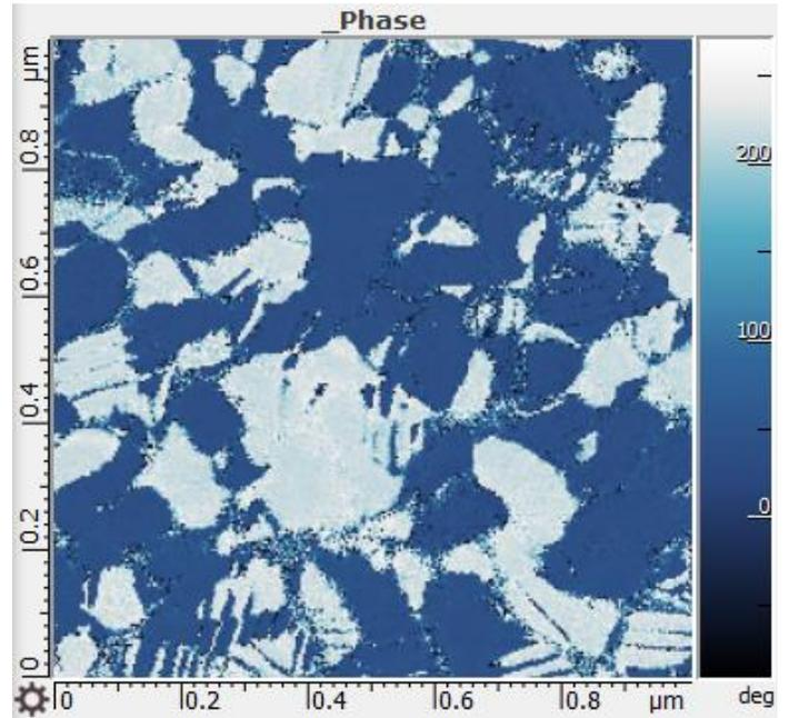
Figure 3: Phase of the vertical piezoelectric response.
