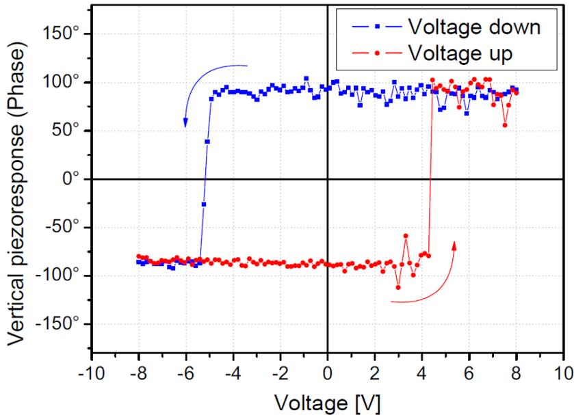
Figure 7: Hysteresis curve of PbTiO<sub>3</sub>. The phase signal changes by 180 degrees when the voltage exceeds a threshold value (coercive field) at about 4 V applied to the tip. This effect is reversible at the negative coercive field.
