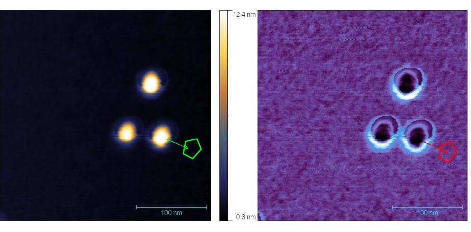
300x300 nm topography (left) and the phase Image of the 14 nm gold nanoparticles from the red circle in previous slide.
