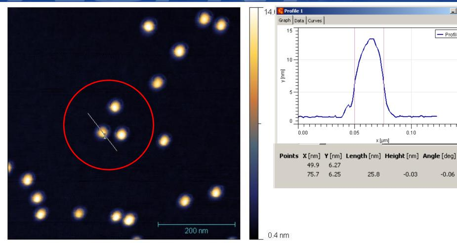
600x600 nm topography image of the 14 nm goldnanoparticles taken with sharp probe. Apparent width a typical nanoparticle is about 26 nm, which is consistent with the 3nm tip radius and the tip's aspect ratio claimed by the probe's manufacturer. Image was obtained in semicontact mode with closed loop in XY-ON.
