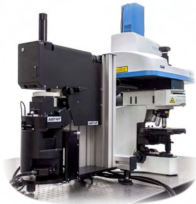
Fig.1 OmegaScope-R coupled with the Horiba XploRAupright Raman spectrometer
